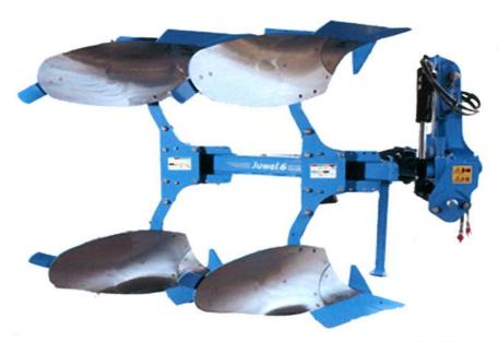
LEMKEN, JUWEL 6 M HYDRAULIC REVERSIBLE TWO BOTTOM MOULD BOARD PLOUGH (Tractor Mounted)
